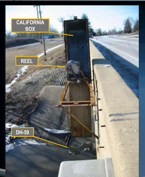
Weekly samples are taken at a fixed location over the thalweg of the main channel using a California-style sediment box that houses a cable, reel, and DH-59 depth-integrated sampler
