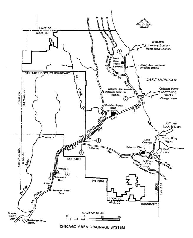
Figure 3. Chicago area drainage system and Lake Michigan diversion inlets
