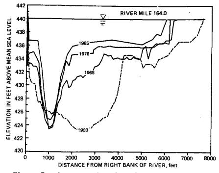
Figure 7. Cross section through lower Peoria Lake at River Mile 164.
