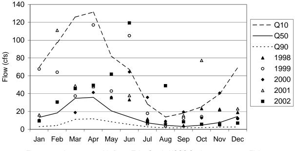
Figure 2.12. Average monthly flows, Tyler Creek, USGS Station 05550300 at Elgin
