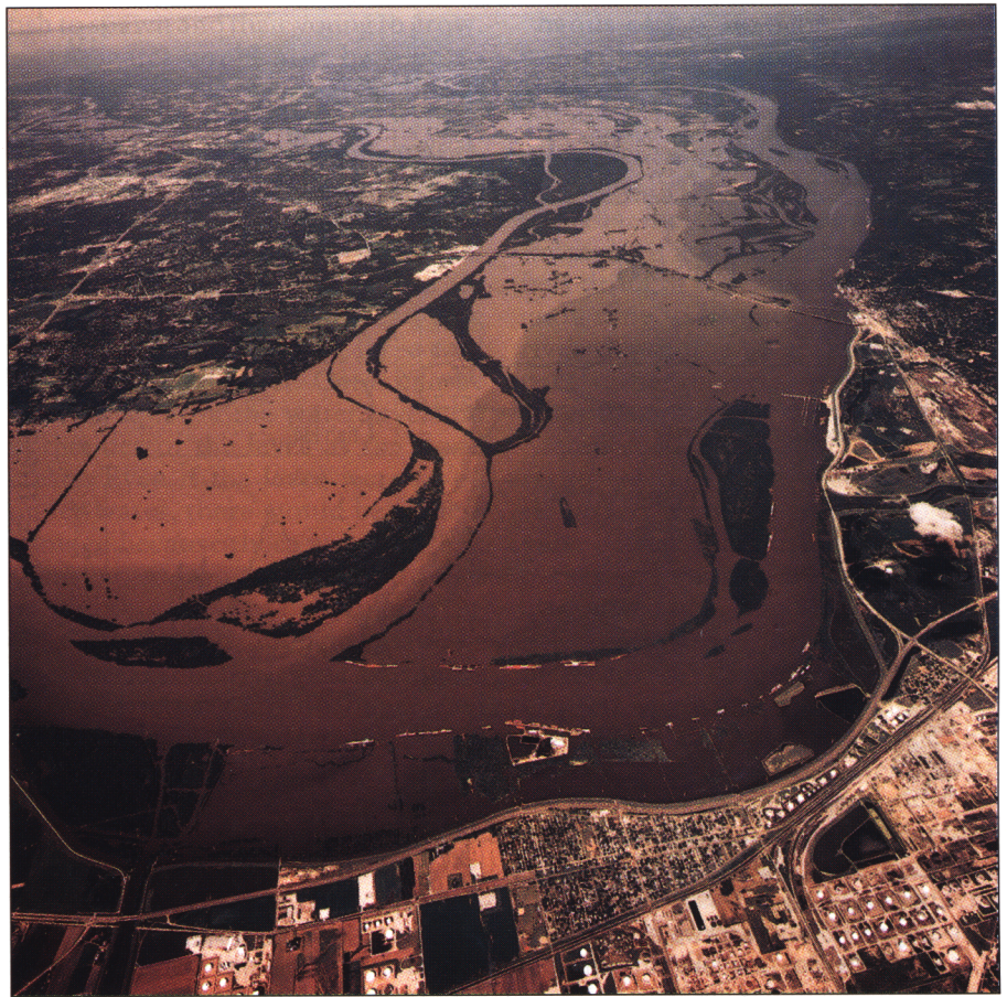
Figure 9. The confluence of the Missouri and Mississippi Rivers just upstream of St. Louis during the 1993 flood. The Missouri is left of center, with the banks delineated by trees; the Mississippi is to the right, with commercial barges tied to the banks. The levee held in Wood River, IL (the city in the foreground). Lock and Dam 26 is just downstream of the bridges visible in the middle distance on the Mississippi at Alton, IL. The lock and gates are visible, but the dam is completely submerged. Some of the water from the Missouri took a shortcut across St. Charles County, MO, into the Mississippi upstream of Dam 26. Photo: Surdex, Inc., St. Louis.
