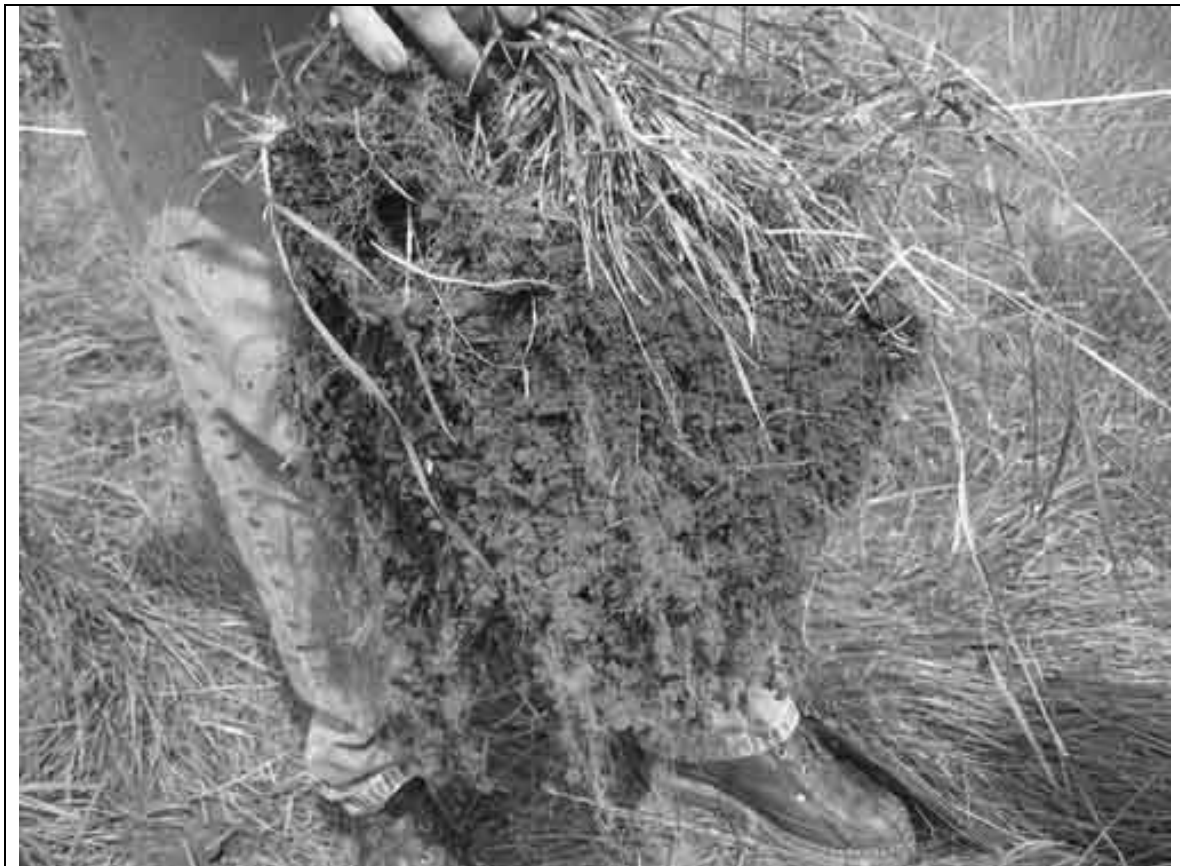
Figure 10. The sediment at the Paxton site rapidly developed granular soil structure and supported healthy vegetation. The pictured grass was planted in March and had no water or fertilizer prior to this photo being taken 4.5 months later.
