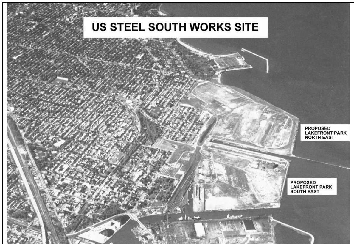
Figure 1. The US Steel Southworks site in Chicago is a prime candidate for using Illinois River sediment as topsoil. The Calumet Channel at the lower right connects to the Illinois Waterway. Barges can carry sediment directly from Peoria Lake to the site of the proposed Lakefront Park South East. This will preclude thousands of trucks hauling soil from suburban development sites over crowded highways and through neighborhoods.
